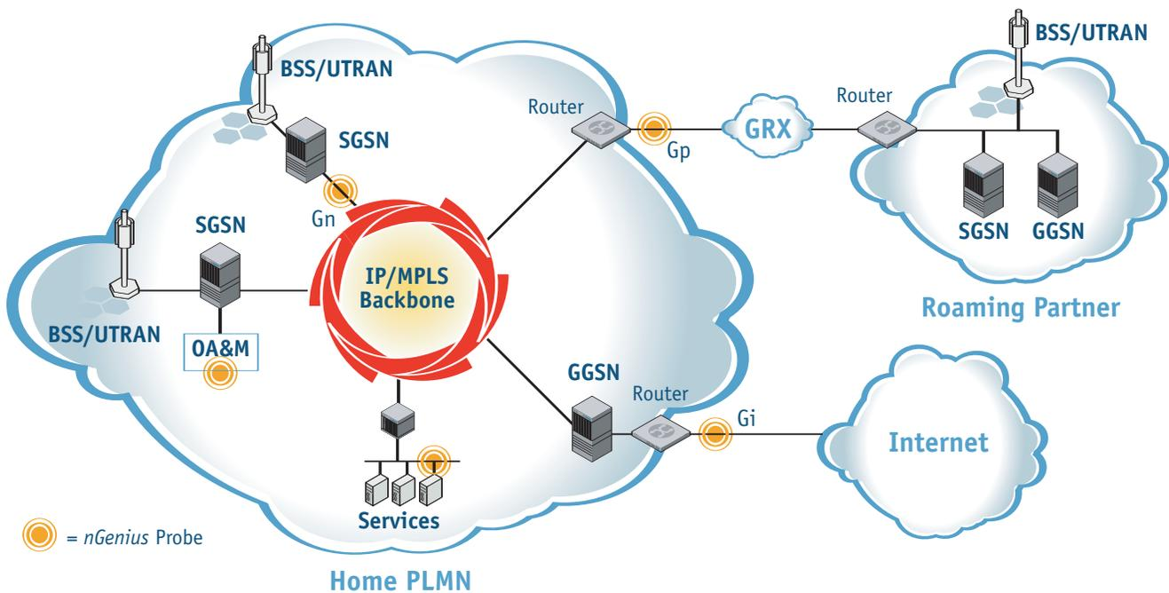
Figure 1. A typical GSM/UMTS network deployment for mobile operations will have base stations, edge routers, access to the public switched telephone network for land line call completion and access to the mobile operator core for completing other cell based calls and delivery of IP-based data services. Shown here are key points where NetScout's *nGenius* Probe and *nGenius* AFMon instrumentation are placed to provide operations performance intelligence.
